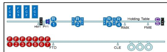
Fig.1. Mill layout of CSC No.1 HSM.
